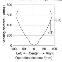
In case using at sensing distance (L3) 500mm, the operation point ( $\ell$ 3) is approx. 81.9mm according to the diagram at left.
