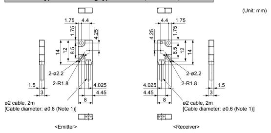
Note: The cable diameter of inflection resistant cable type is Ø0.7mm.
