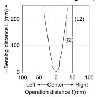
In case using at sensing distance (L2) 200mm, the operation point ( $\ell$ 2) is approx. 30.5mm according to the diagram at left.
