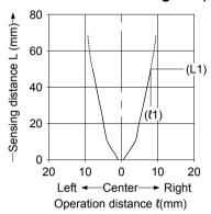
In case using at sensing distance (L1) 50mm, the operation point ( $\ell$ 1) is approx. 8.02mm according to diagram above.
