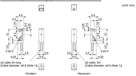
Note: The cable diameter of inflection resistant cable type is ø0.7mm.
